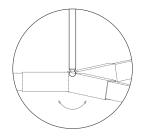
All Bough fixtures feature a 0-15° adjustable ball swivel that allows fixtures to be configured in different angles.
