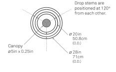
Double Chime Cascade (CSCD-M3-L3) consists of one Middle Chime (3ft) and one Little Chime (3ft). Alternate combinations available upon approval.
