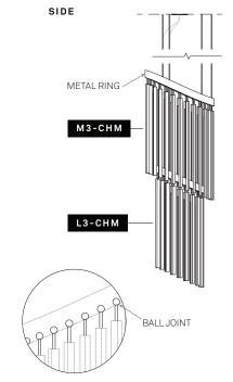
All Chime fixtures feature a 360° BALL JOINT that allows each bulb to rotate within its socket.
