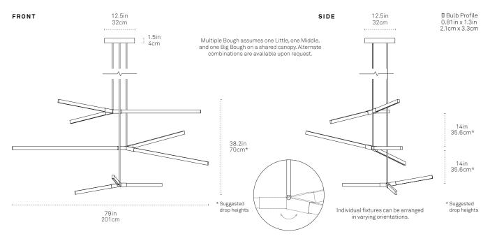
All Bough fixtures feature a 0–15° adjustable ball swivel that allows fixtures to be configured in different angles.
