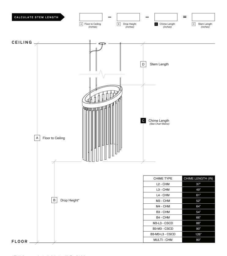
\* Stickbulb recommends using the highest possible 'Drop Height.' We will include 3 additional segmented stem sets in 2" increments. This will allow you to drop the fixtures between 2" to 6" lower. \*\* Note: each ring requires separate AC input + dimming control
